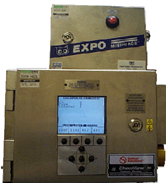
Simulplex™ ChemView® in Class 1, Div 2 Z-Purged Enclosure for Two Probes
